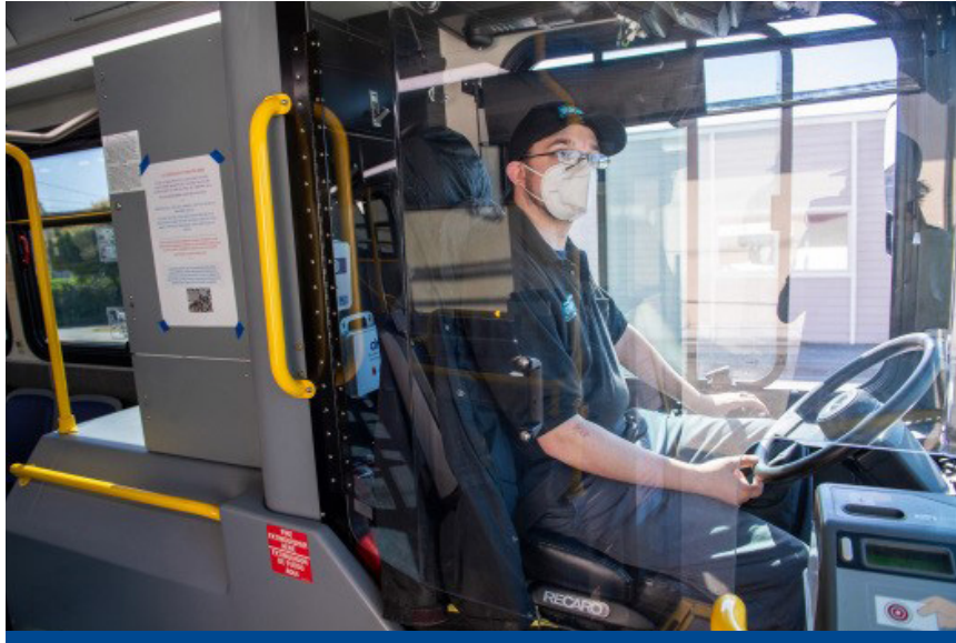
A plexiglass shield separates a bus driver from passengers on a Humboldt Transit Authority vehicle. Source: The Times Standard
