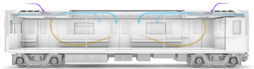
The New York City subway systems exchanges its air 18 times/hour, well above the recommended flow rate for many other indoor settings. (Image source: The New York Times)
